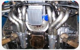
All our headers are made from mandrel bent tubing and TIG welded. Not only do they flow well
